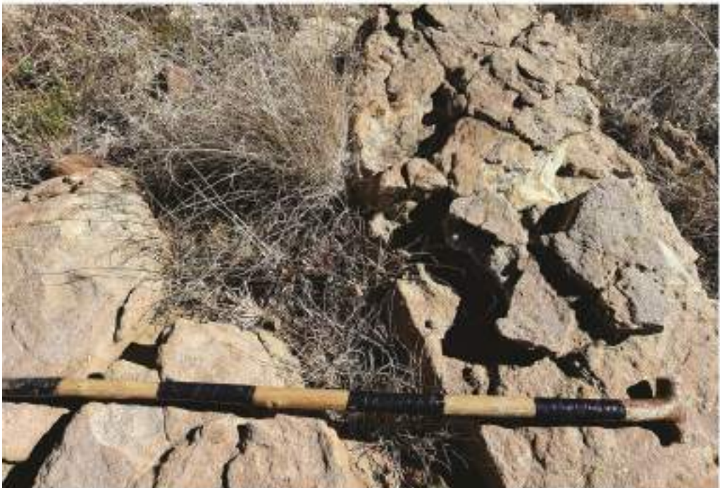
Figure 8. Intact, coarse-grained Molteno Formation sandstone outcropping to the west, south and east of the existing borrow pit. Scale 1 = 10 cm.
