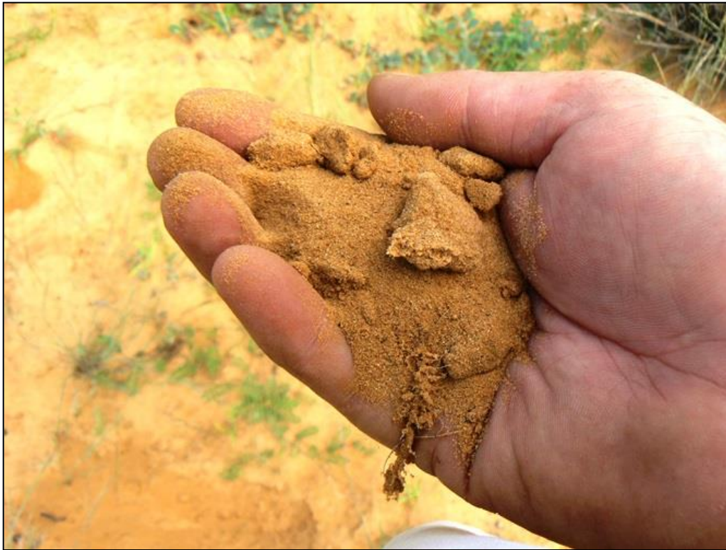
Photograph 4. Sandy nature of the red Aeolian sands associated with the Hutton soil form
