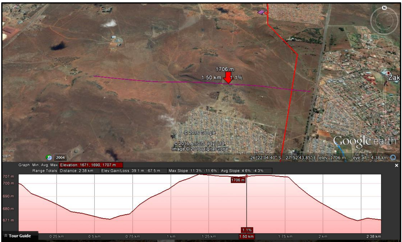
Figure 9: East-west elevation profile of a section of Class 1 ridge along the proposed route (maximum slope 11.3%).
