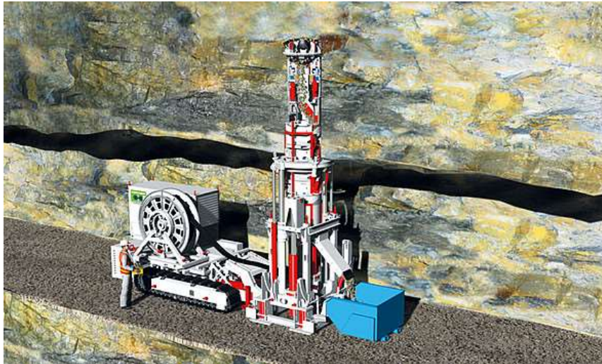
Figure 13 | Illustration of the raise bore method.
