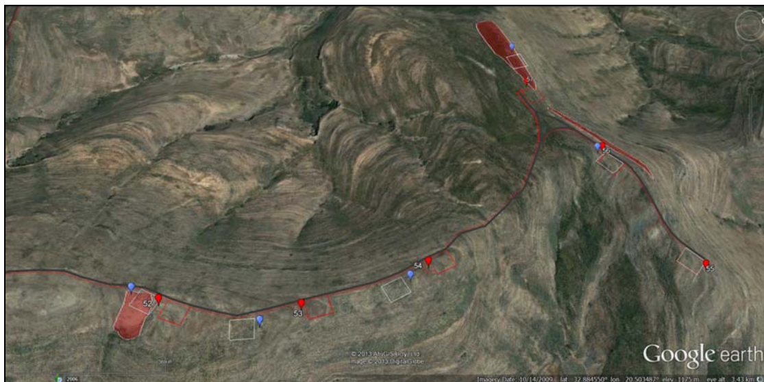
Figure 11.2 Satellite image illustrating the turbines that were relocated on the basis of the assessment of the final development layout. The blue markers illustrate the original location of the turbines, while the red markers show the revised locations. The red polygons illustrate the sensitive areas that were observed and mapped in the field.
