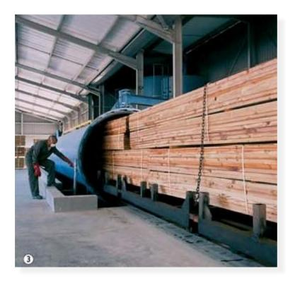
Figure 3: Example of a Tanalith® C treatment vessel (Tanalised® C)
