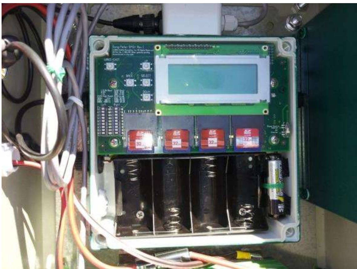
Figure 3: SM2BAT+ detector with four 32 GB SDHC memory cards.
