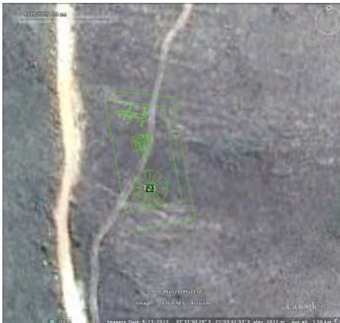
Figure 2-2: An example of a turbine footprint, including the turbine and laydown areas used during construction.
