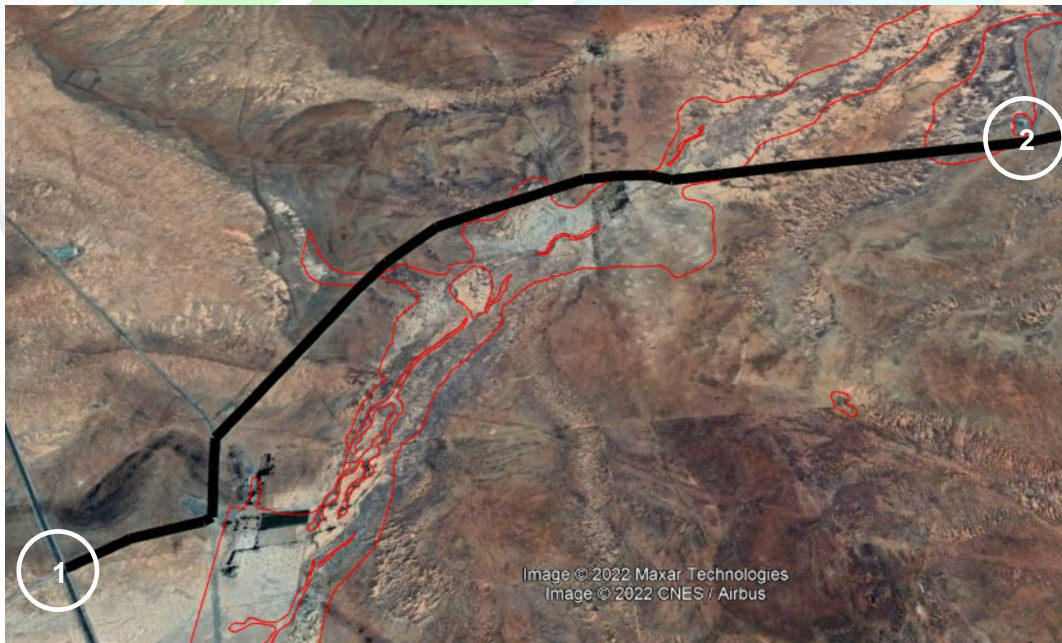
Figure 3. Section of existing public 'Burgerville' District Road (2448) from its intersection with the N10 (1) to its intersection with the existing private road (farm track) at the boundary of Farm Riet Fountain 39C (2). Red lines indicate flood plain soils (possible watercourses).
