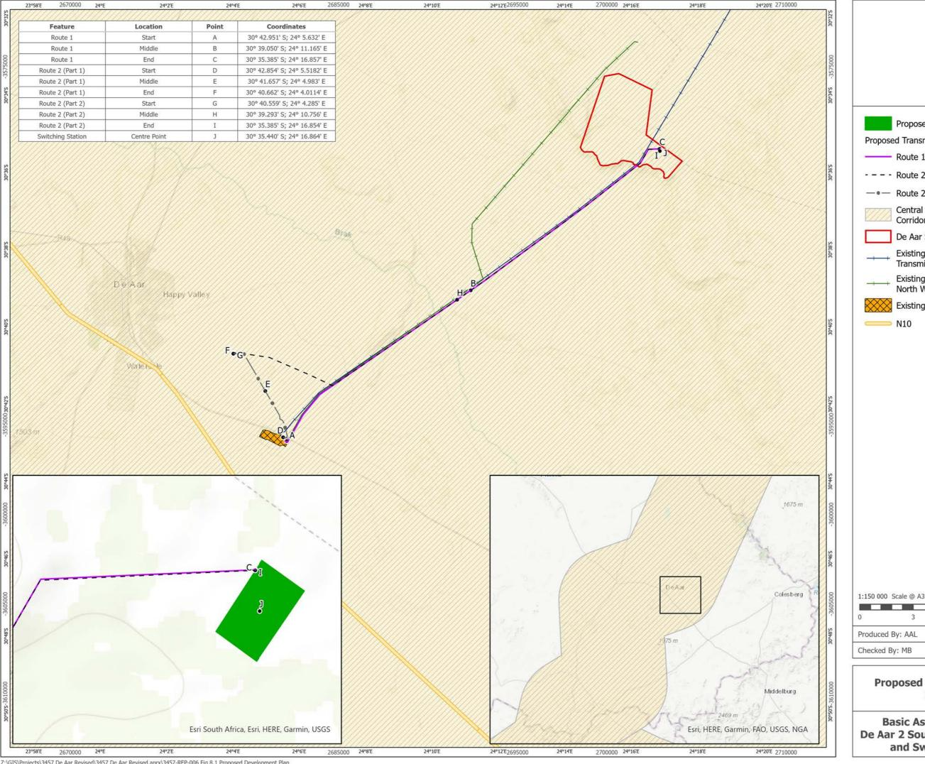
**S**ARCUS Proposed Switching Station Proposed Transmission Lines Route 1 (Preferred Alternative) - Route 2 (Part 1) (Alternative 1) —●— Route 2 (Part 2) (Alternative 1) Central Strategic Transmission Corridor De Aar South WEF Existing Hydra Roodekuil 220kV Transmission Line Existing Longyuan Mulilo De Aar 2 North WEF Transmission Line Existing Eskom Hydra Substation 1:150 000 Scale @ A3 6 km Ref: 3457-REP-006 Date: 2021/03/12
