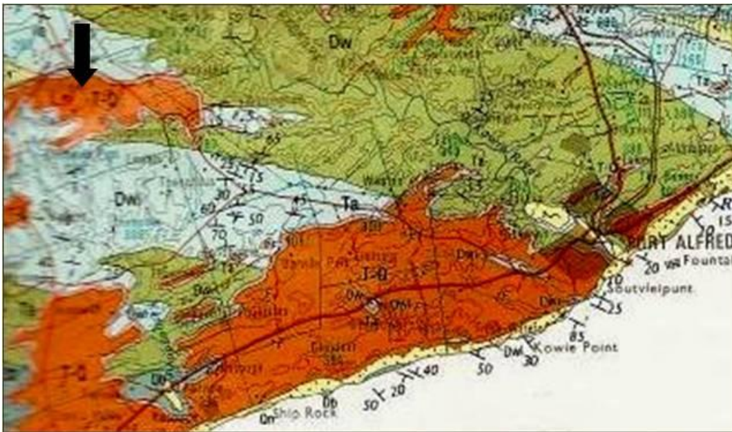
Figure 18: General geology of the area: The Nanaga Formation is mapped in brown with the symbol “T-Q”. The Witpoort Formation is mapped in light blue with the symbol “Dwi” which is underlain by the Weltevrede Formation comprising shale and subordinate quartzite (sandstone) layers and is mapped in khaki-green with the symbol “Dw”. Both of these formations are of the Witteberd Group, Cape Supergroup.
