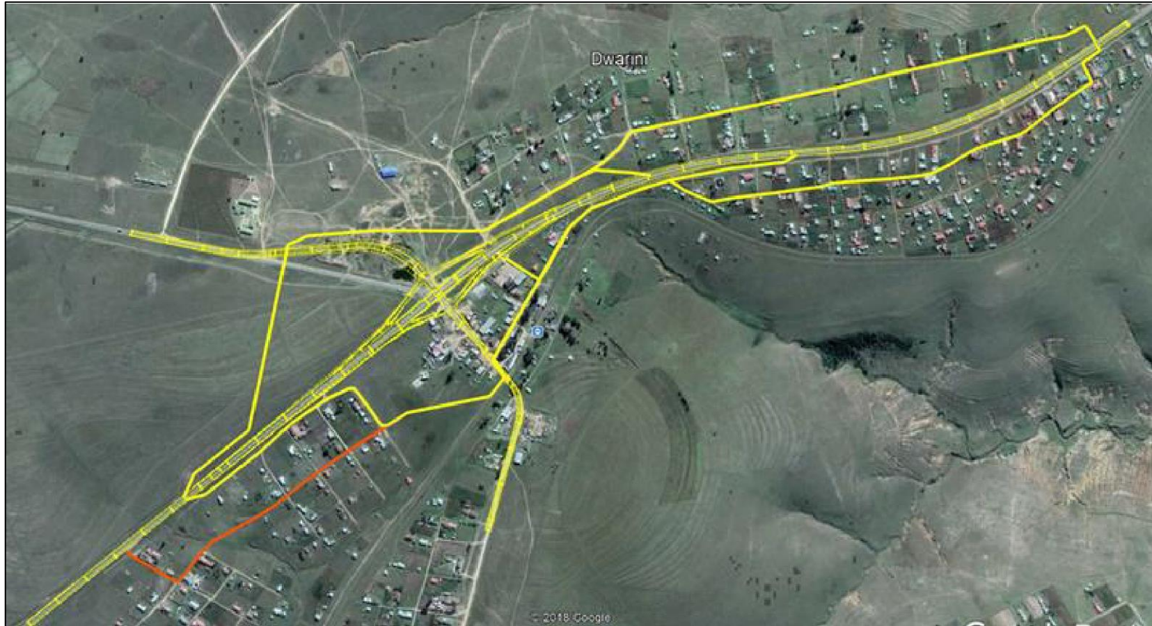
Figure 1-3: Aerial representation of the Ndabakazi Interchange Upgrade infrastructure components as discussed in the text. An alternative temporary route is indicated in orange.
