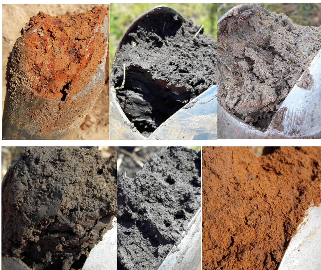
Figure 10-4: Examples of soils found on the Vaalkop site (Glencoe, Rensburg, Longlands, Bonheim, Arcadia and Hutton, respectively)
