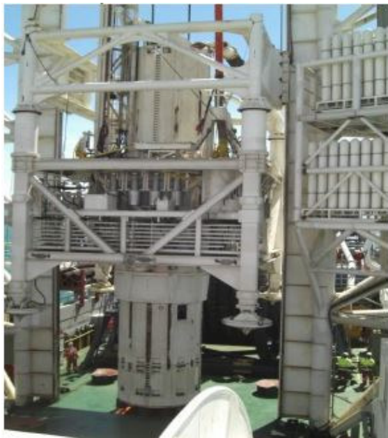
Figure 2: Illustrative example of a drill bit operated from a drill frame structure located onboard a vessel of opportunity.
