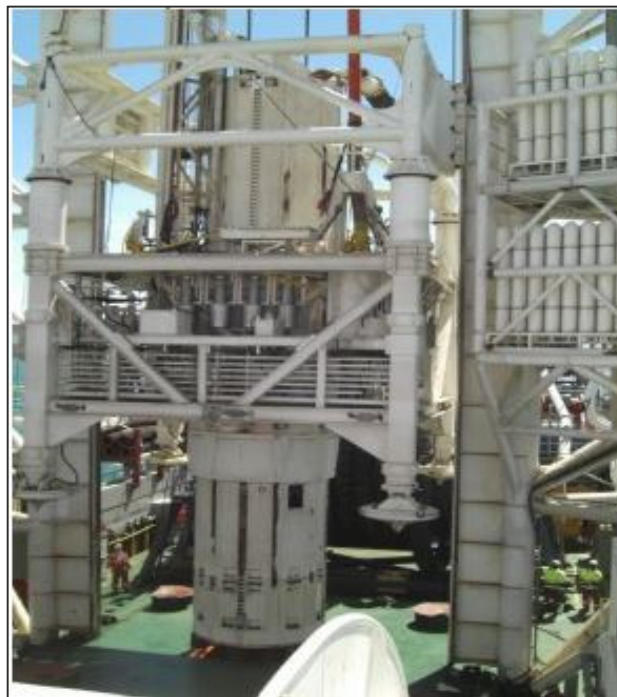
FIGURE 3-4: ILLUSTRATIVE EXAMPLE OF A DRILL BIT OPERATED FROM A DRILL FRAME STRUCTURE LOCATED ON BOARD A VESSEL OF OPPORTUNITY.
