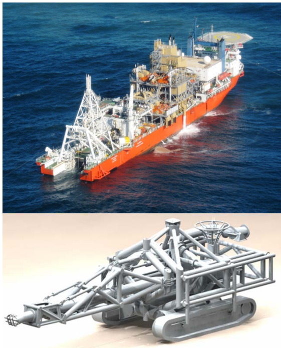
Figure 2: mv Peace in Africa mining vessel, representation of horizontal mining and illustration of the seabed crawler.
