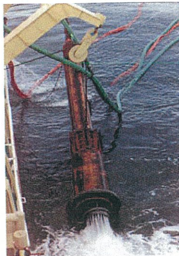
FIGURE 5: Standard skirted megadrill (0.72m 2 ) using airlift system principal
