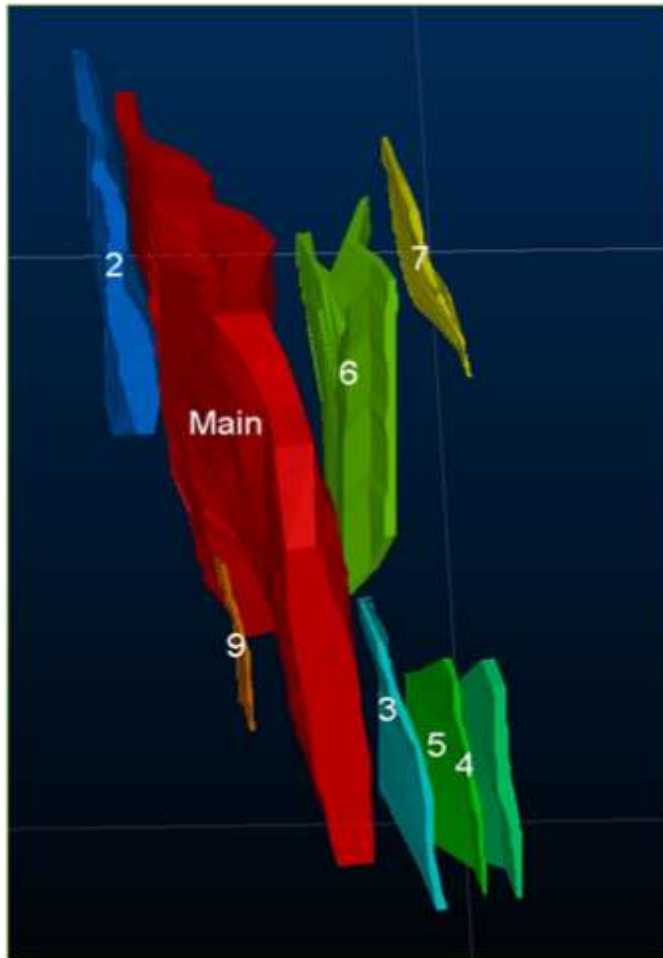
Figure 4. Section view of the Witkop open-pit Mineral Resource showing the different zones of mineralisation Viewed from the East
