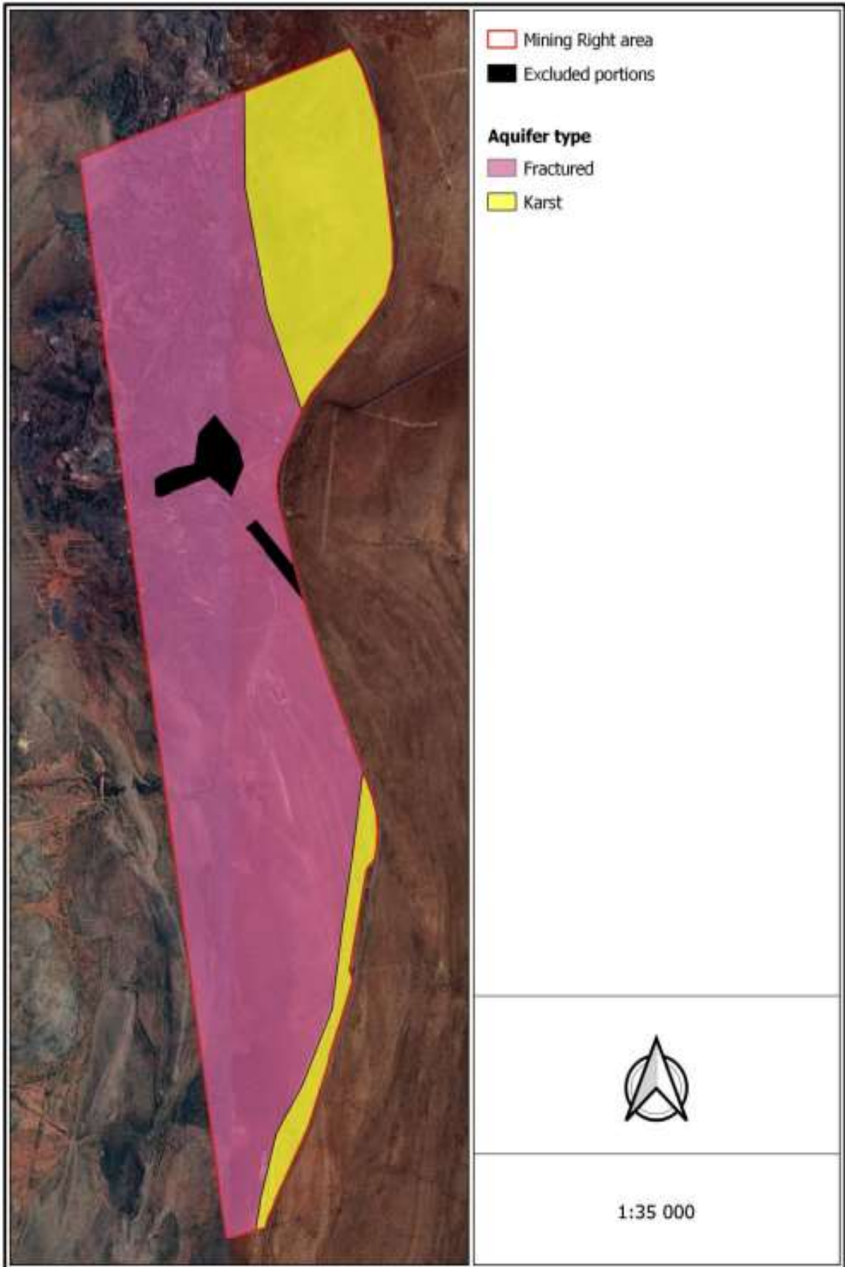
Figure 15. The location of aquifer systems in relation to the proposed mining right area.
