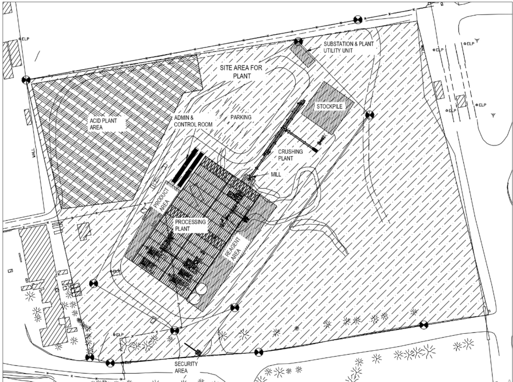
Appendix A: Layout map of the preferred development footprint for the zero waste recovery plant, as was assessed as part of the EIA process
