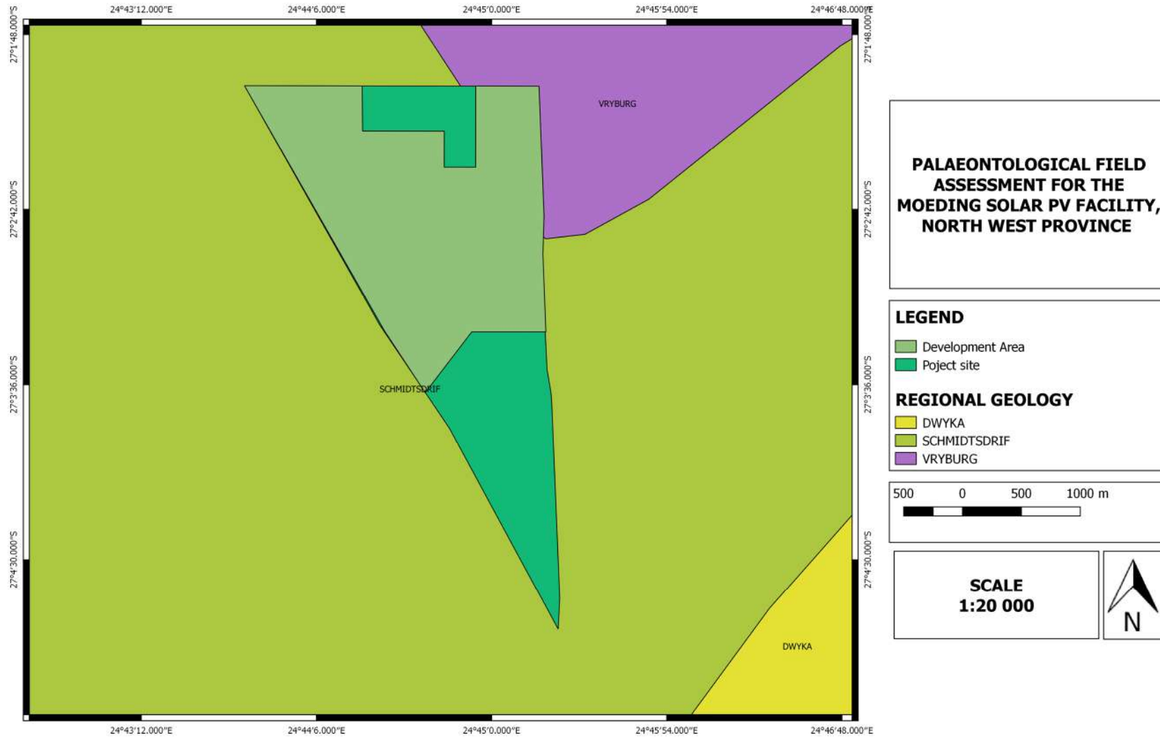
Figure 6.9: The surface geology of the proposed project site. The site is underlain by the Vryburg Formation (Transvaal Supergroup) and the Schmidtsdrif Subgroup, Ghaap Group of the Transvaal Supergroup.
