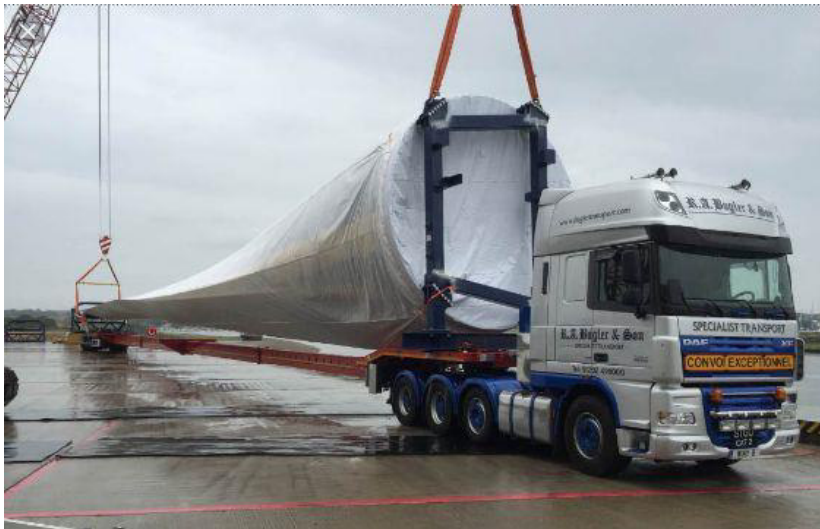
Figure 2.2: Example -Transport of Blades on extendible trailers
