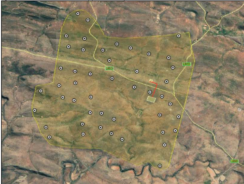
Figure 2: Aerial view of the development envelope indicating the proposed wind turbine layout (white dots), substation site (yellow rectangle) and power line (red line).
