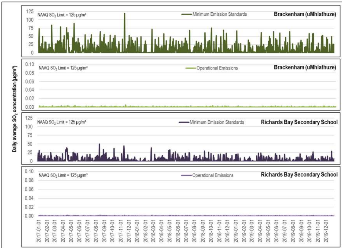
Figure 7-2: Time series of the daily SO 2 concentrations simulated at the nearest AQMS and receptor
