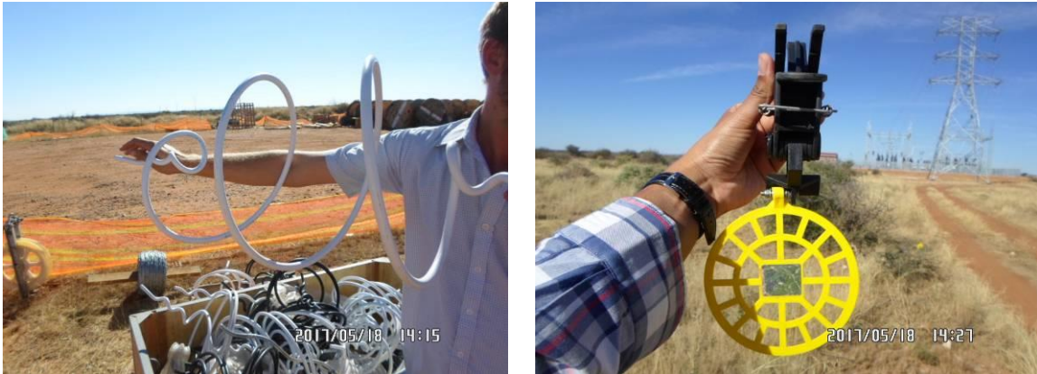
Figure 277: Examples of bird flight diverters to be used on the power lines: Double loop bird flight diverter (left) and Viper live bird flapper (right).
