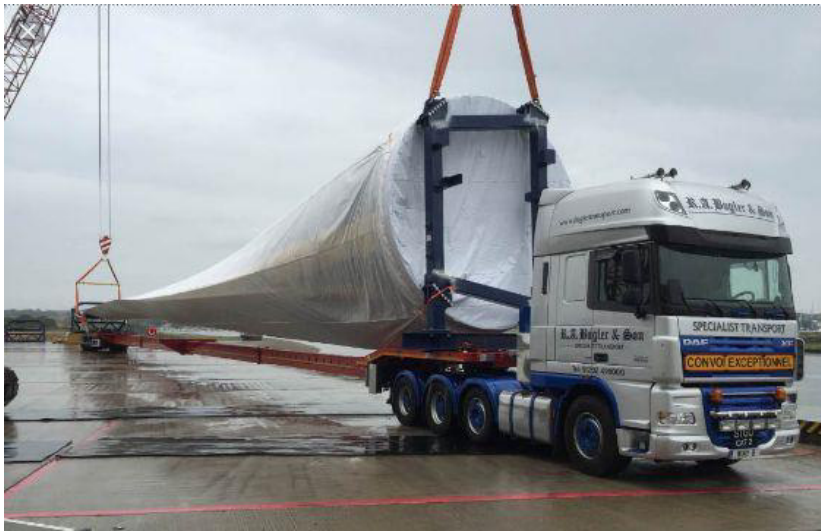
Figure 2-2: Example -Transport of Blades on extendible trailers
