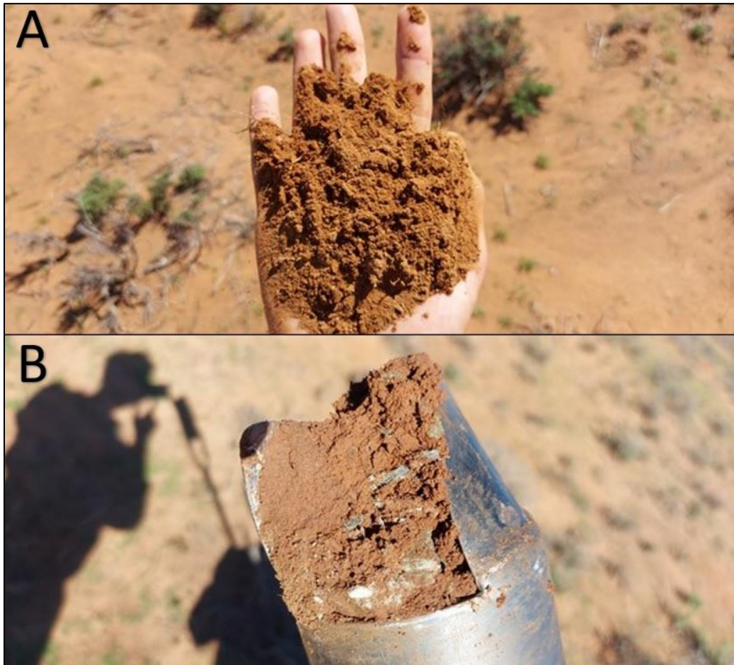
Figure 6-1 Examples of soil horizons identified on-site. A) Neocutanic horizon. B) Transition between neocutanic and lithic horizon
