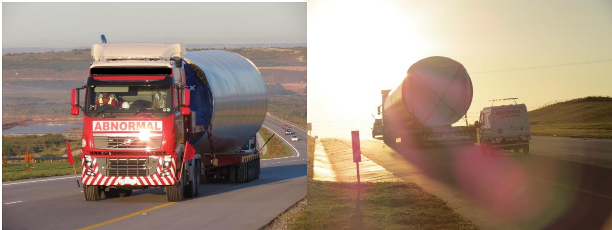
Figure 2-4: Example – Transportation of Tower Sections
