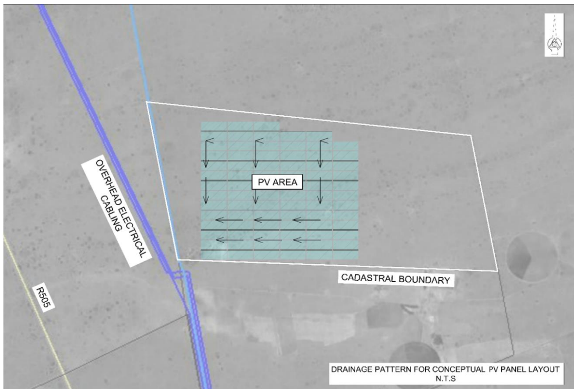
Figure 4.2: Drainage pattern for conceptual layout of PV panels
