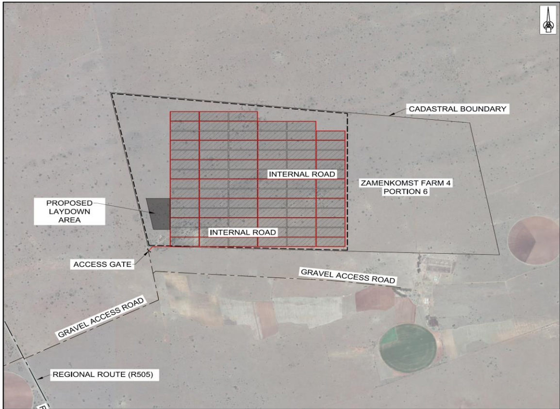
Figure 4.1: Conceptual Layout of PV Panels
