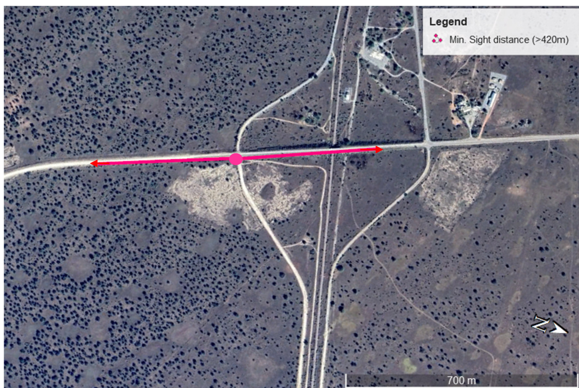
Figure 4-18: Required Sight distance at R385 / Gravel Road
