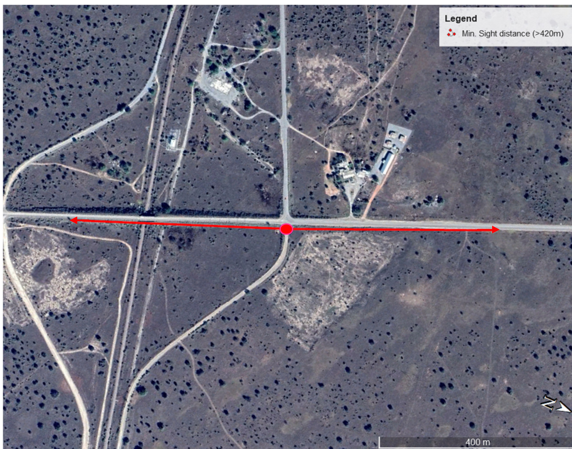
Figure 4-11: Required Sight distance at R385 / gravel road
