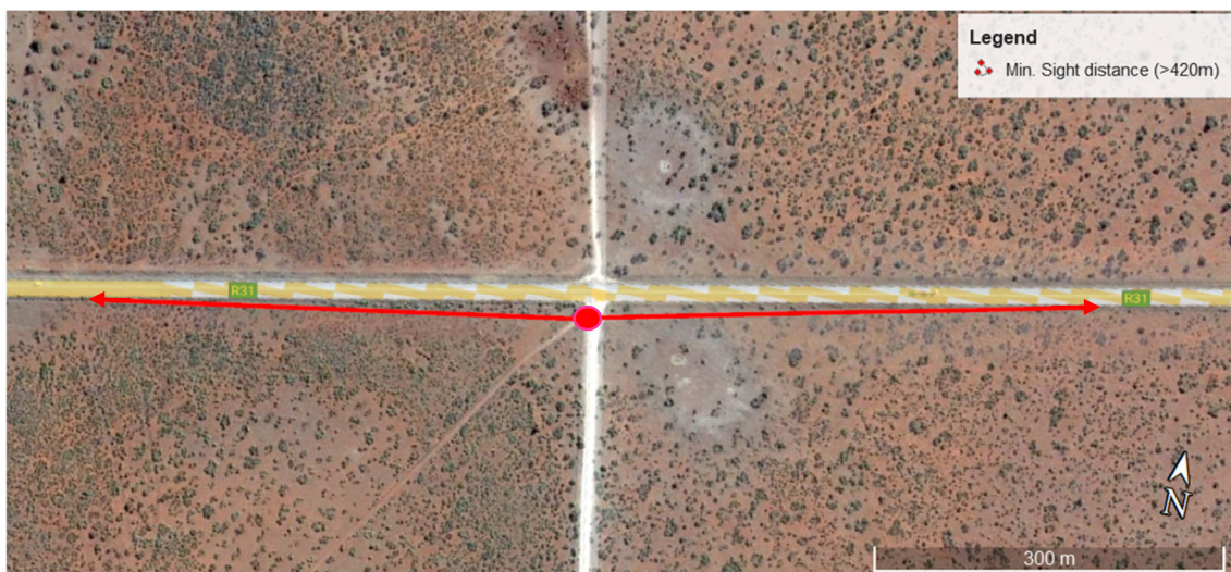
Figure 4-6: Required Sight distances at R31 / Gravel road
