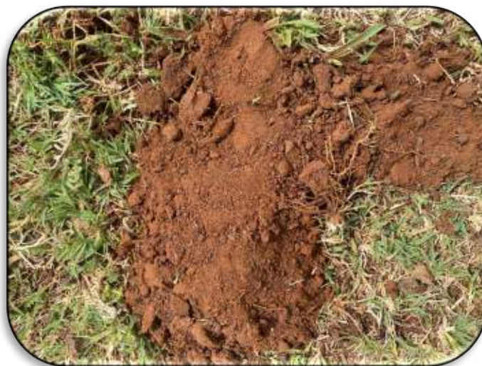
Figure 4: Orthic, red apedal B, unspecified, Hutton soils sampled within the proposed footprint of Seelo Alpha Solar PV
