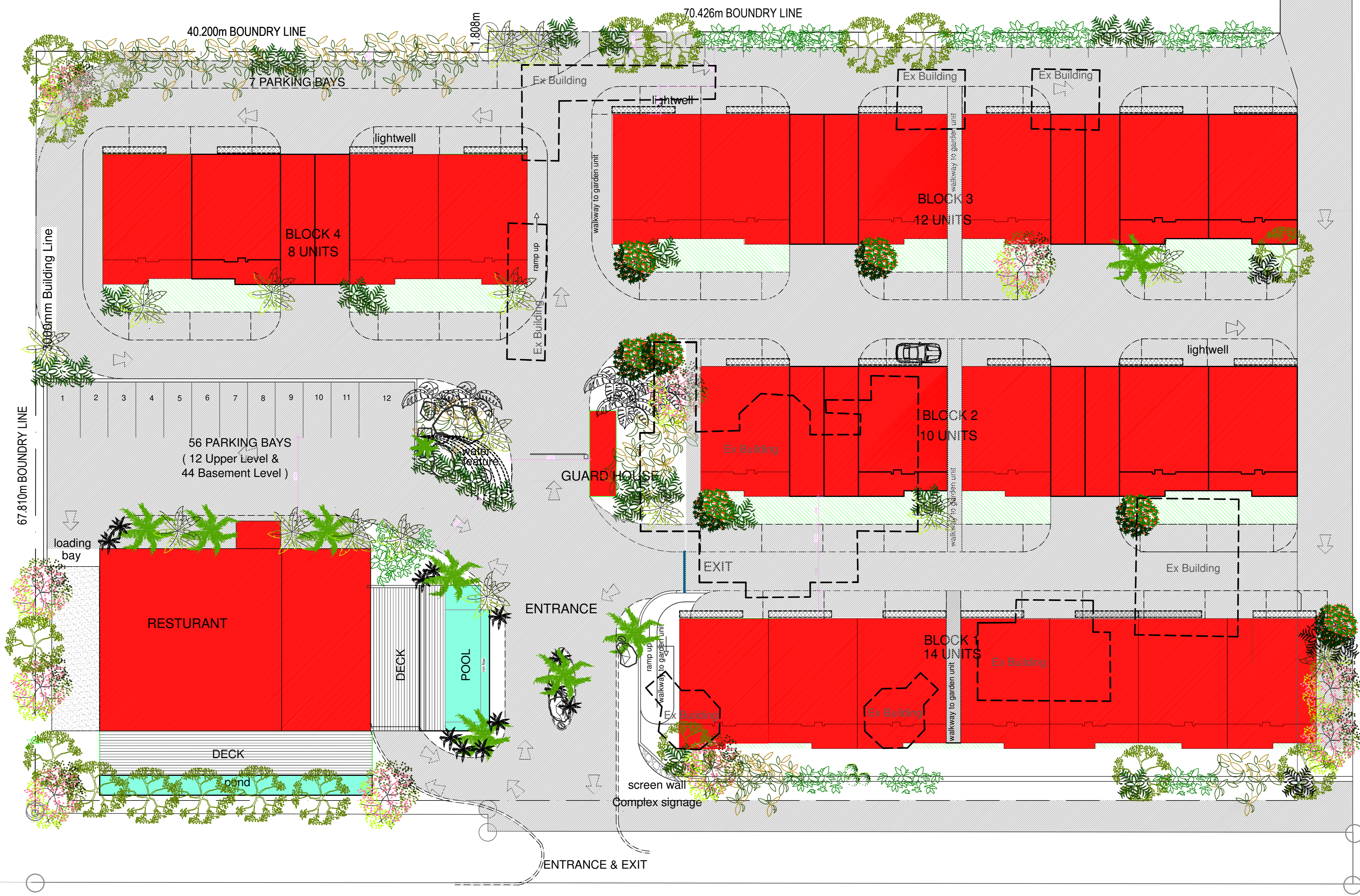
SITE PLAN - DEVELOPMENT PROPOSAL WITH OVERLAY OF EXISTING BUILDINGS TO BE DEMOLISHED
