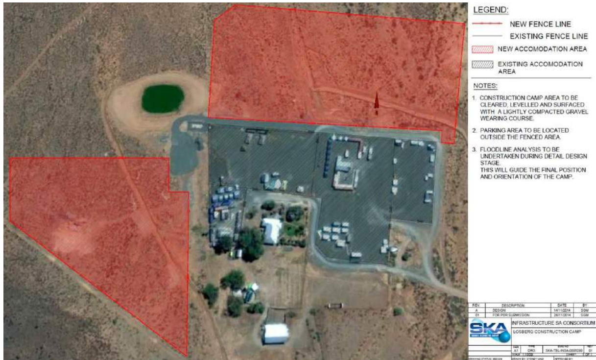
Figure 2-26: New accommodation area at the Losberg construction camp
