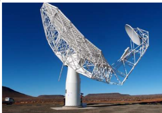
Photo 6: MeerKAT antenna on a foundation
