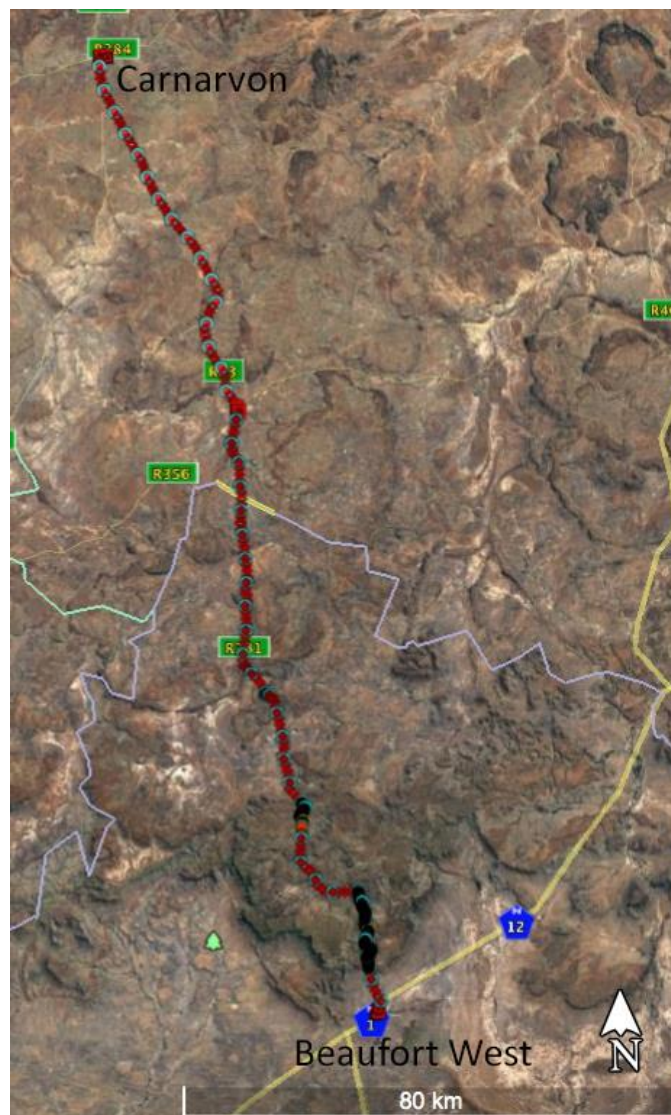
Figure 37: Map indicating the overhead sections (black dots) and the trench sections (red).
