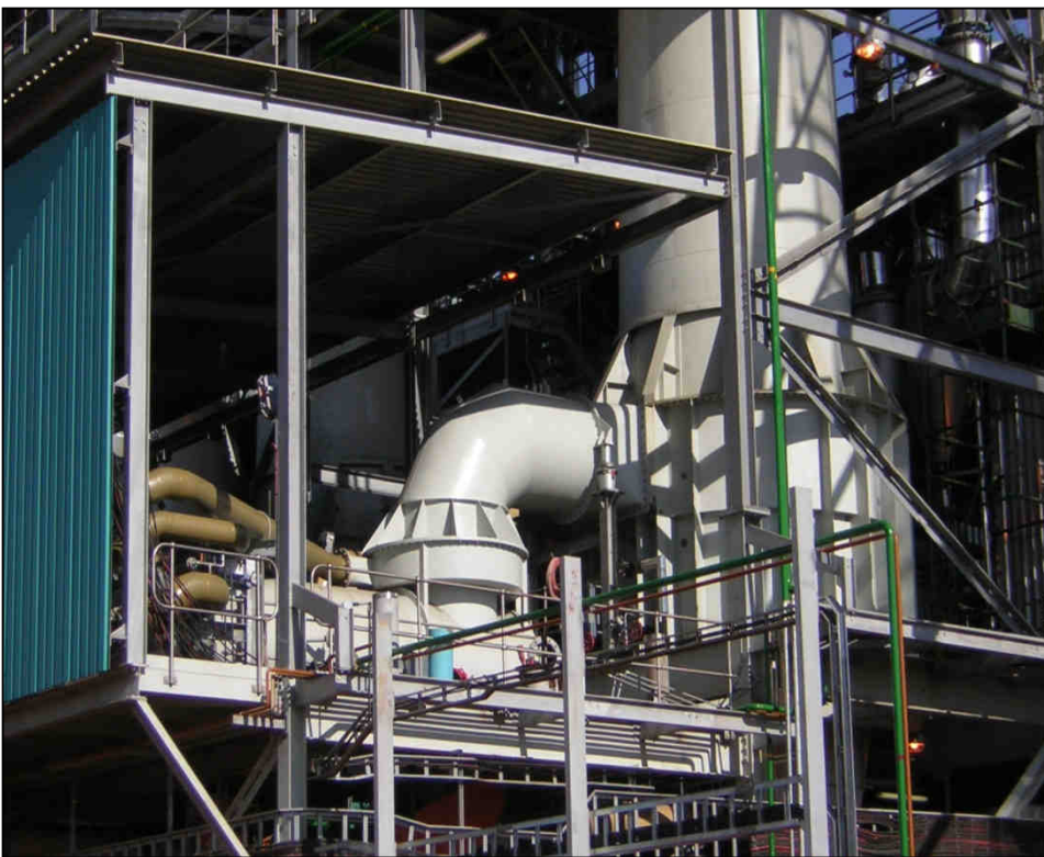
Plate 2.11: The retort in which the coal is heated.
