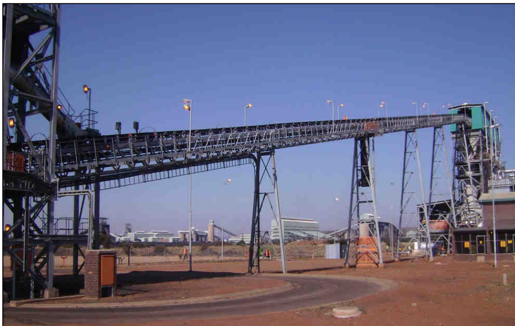
Plate 2.9: The screened coal is transported via conveyor belt to the retort feed bins located above the retorts.
