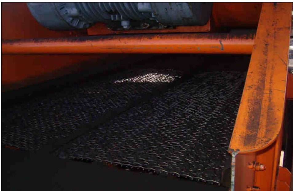
Plate 2.8: The vibrating screen – coal is passed over this screen to remove the unwanted fines less than 15 mm in size.
