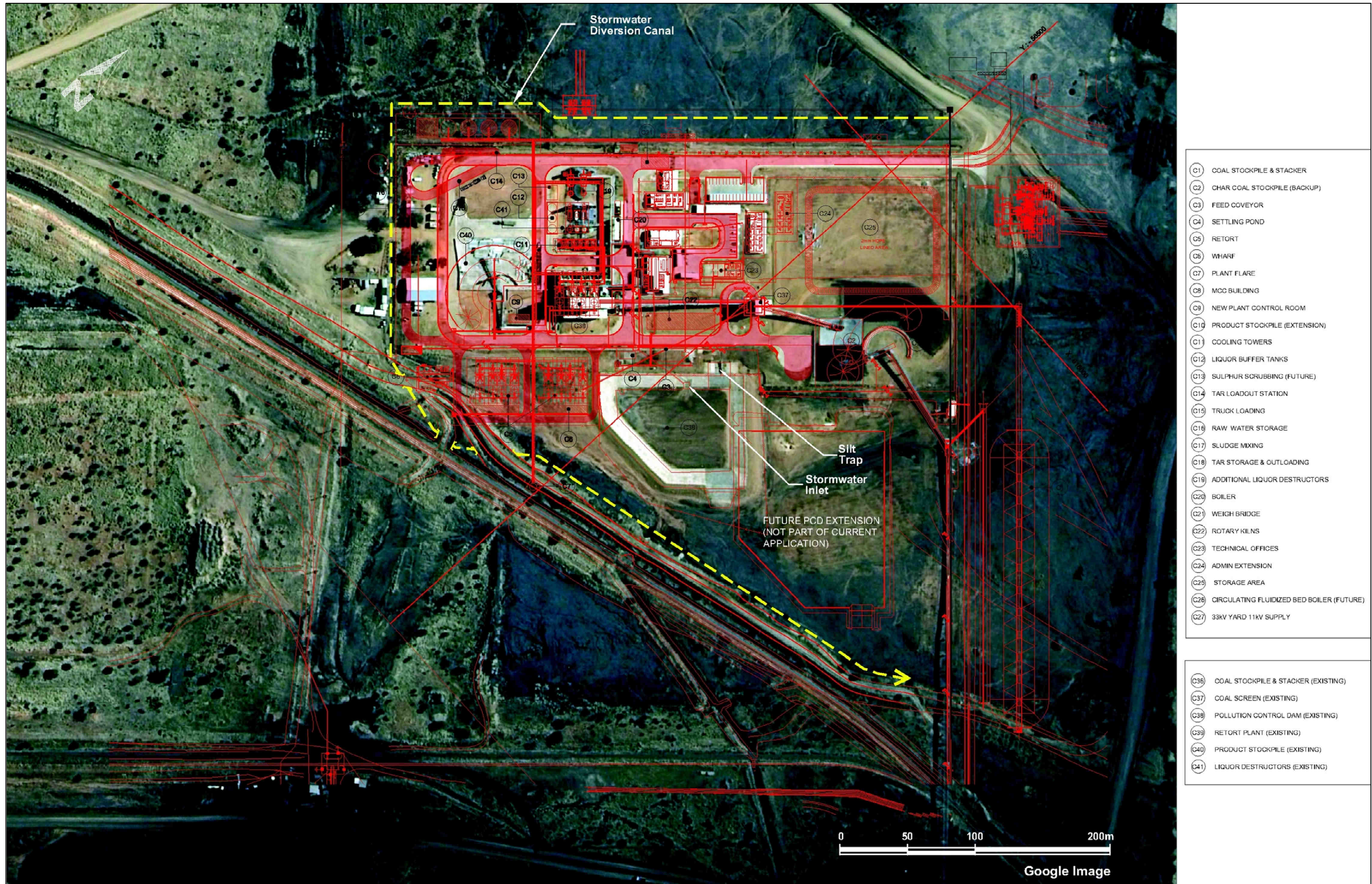
Figure 6.9: Layout of the storm water management system (showing the stormwater cut-off drain) for the Char Manufacturing Plant Expansion
