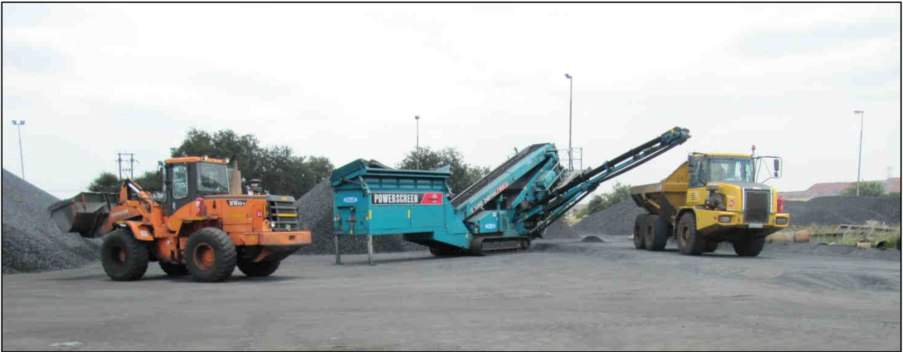
Plate 2.14: Char is stockpiled and separated (screened) into char fines and lumpy char.
