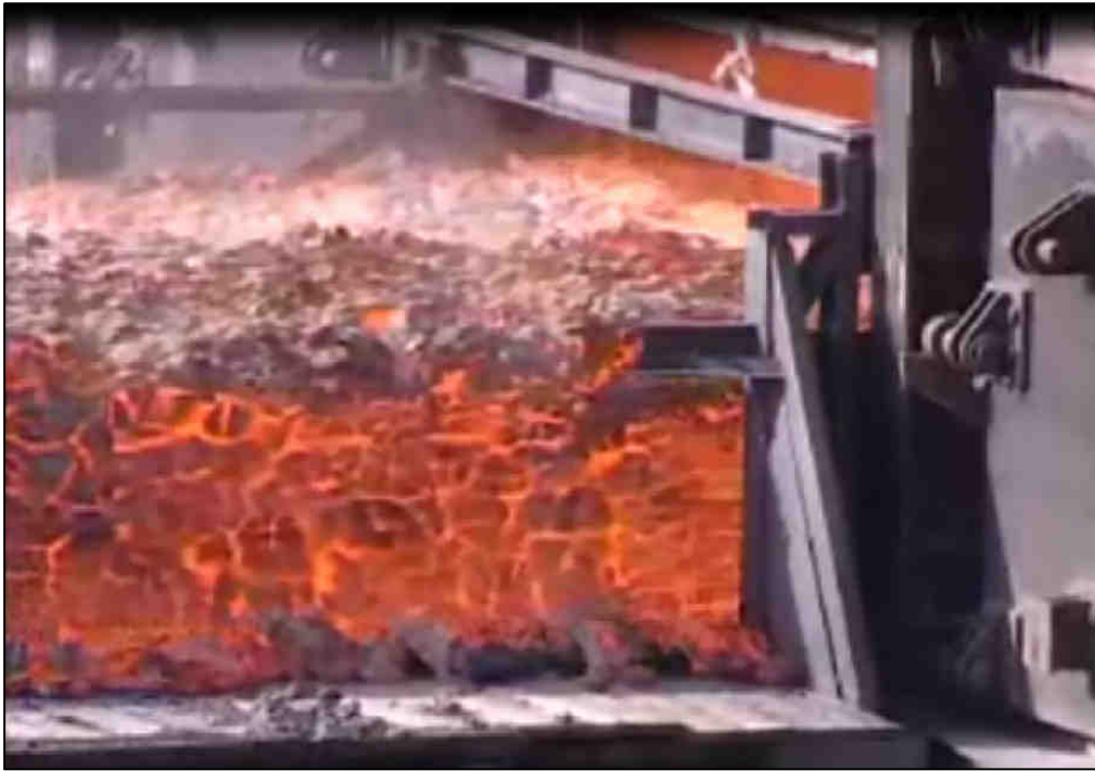
Figure 2.5: A coke cake which has been heated and is being pushed out of the coke oven (Courtesy Sinosteel).
