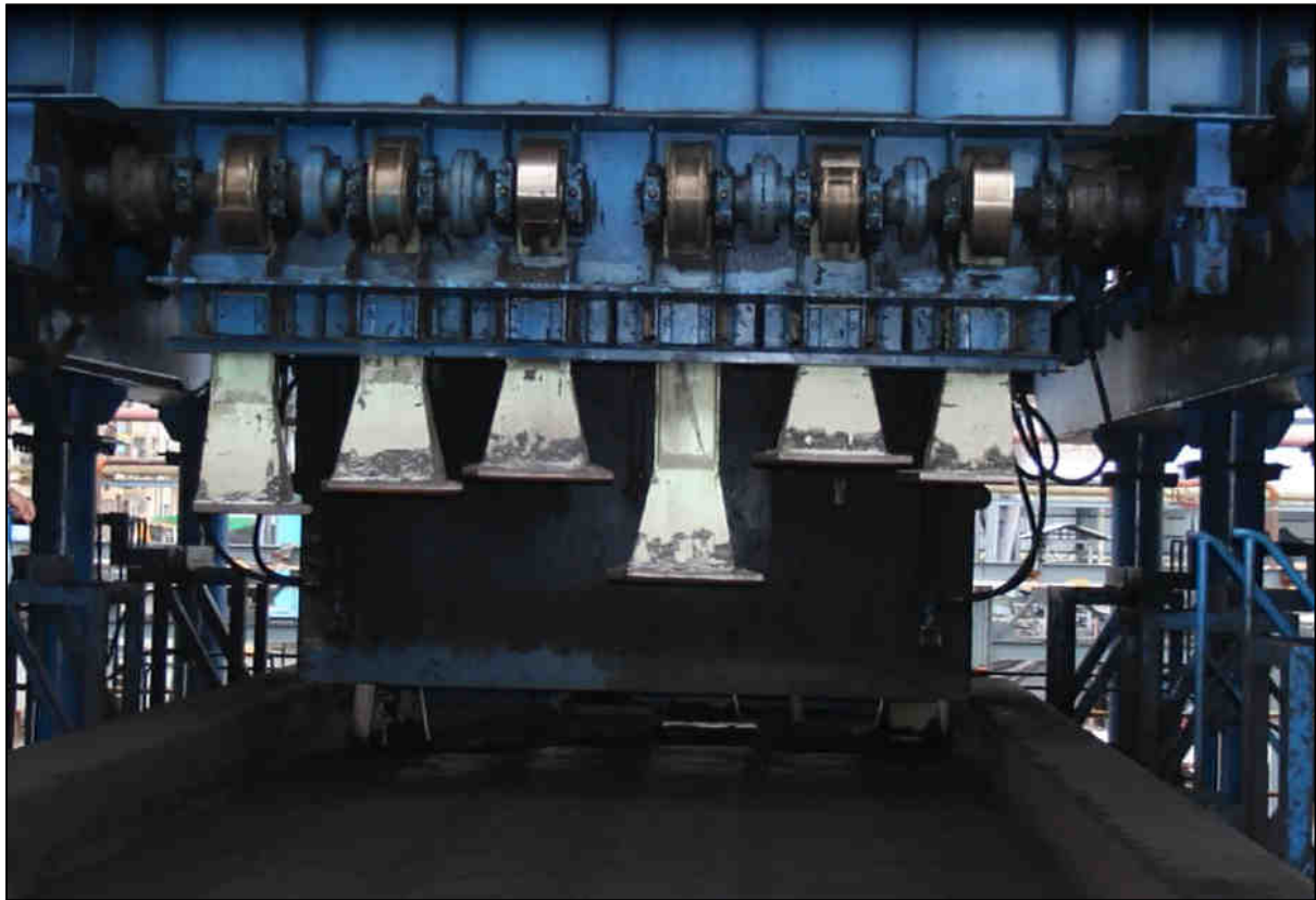
Figure 2.2: Coal cake being compressed by stamping machine (Courtesy Sinosteel)
