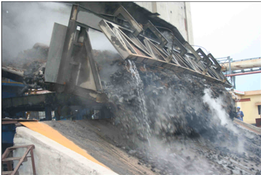
Figure 2.10: Discharging quenched coke on to a coke wharf (similar to proposed Market Coke Plant) (Courtesy Sinosteel).
