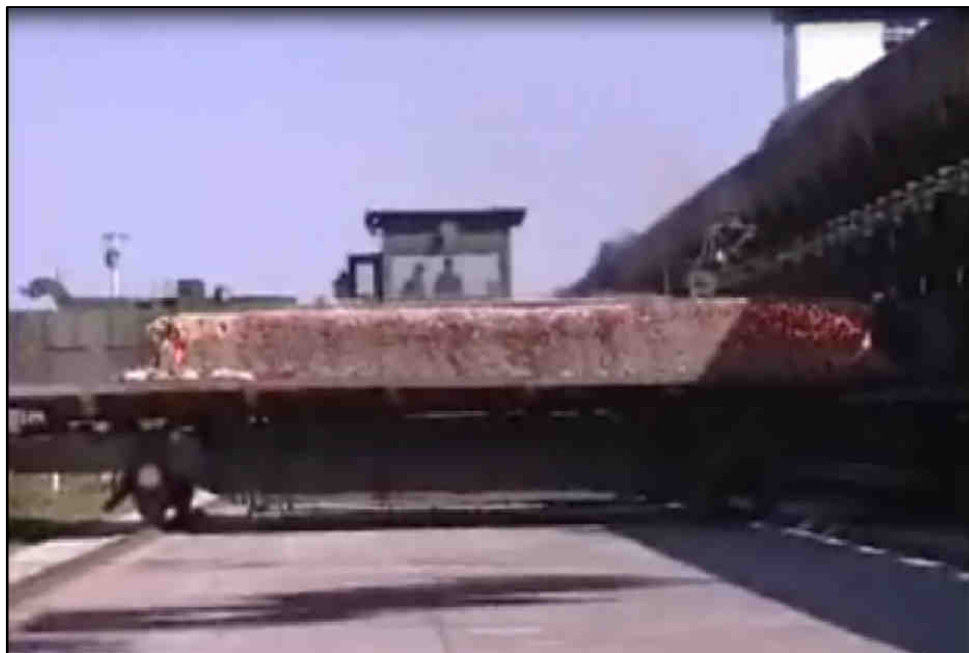
Figure 2.6: A coke cake which has been pushed out of the coke oven onto the quenching car (Courtesy Sinosteel).
