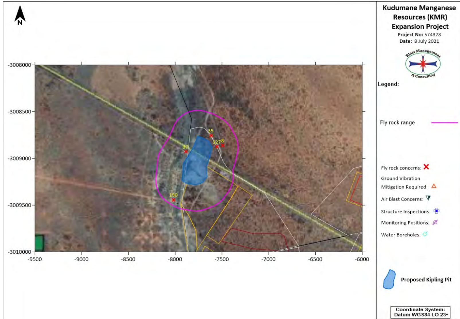
Figure 27: Predicted Fly Rock Exclusion Zone for the Kipling Pit area
