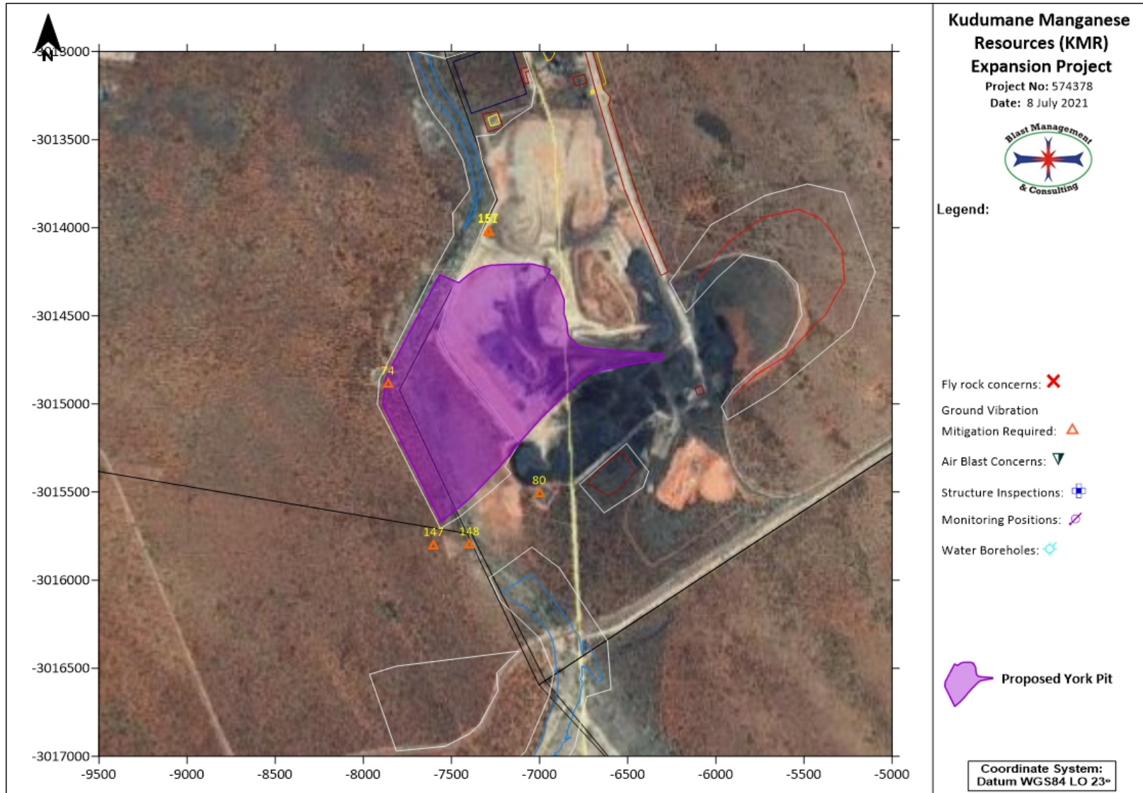
Figure 28: Structures identified where ground vibration mitigation will be required – York Pit
