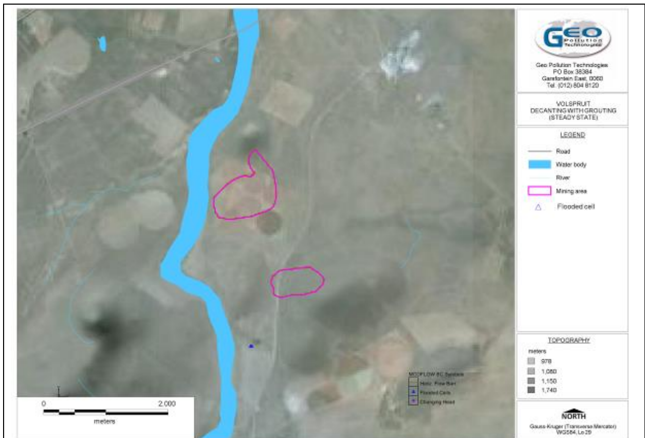
Figure 8-32: Post mining opencast pit decant (With clay barrier / grouting installed)
