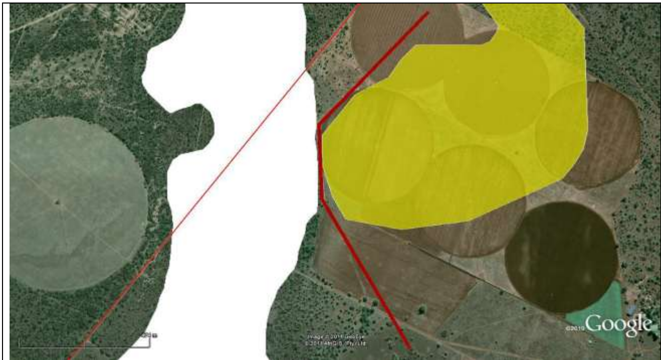
Figure 9-2: Proposed position of flood barrier wall (indicated as thick red line between North Pit (yellow) and wetland (white)).
