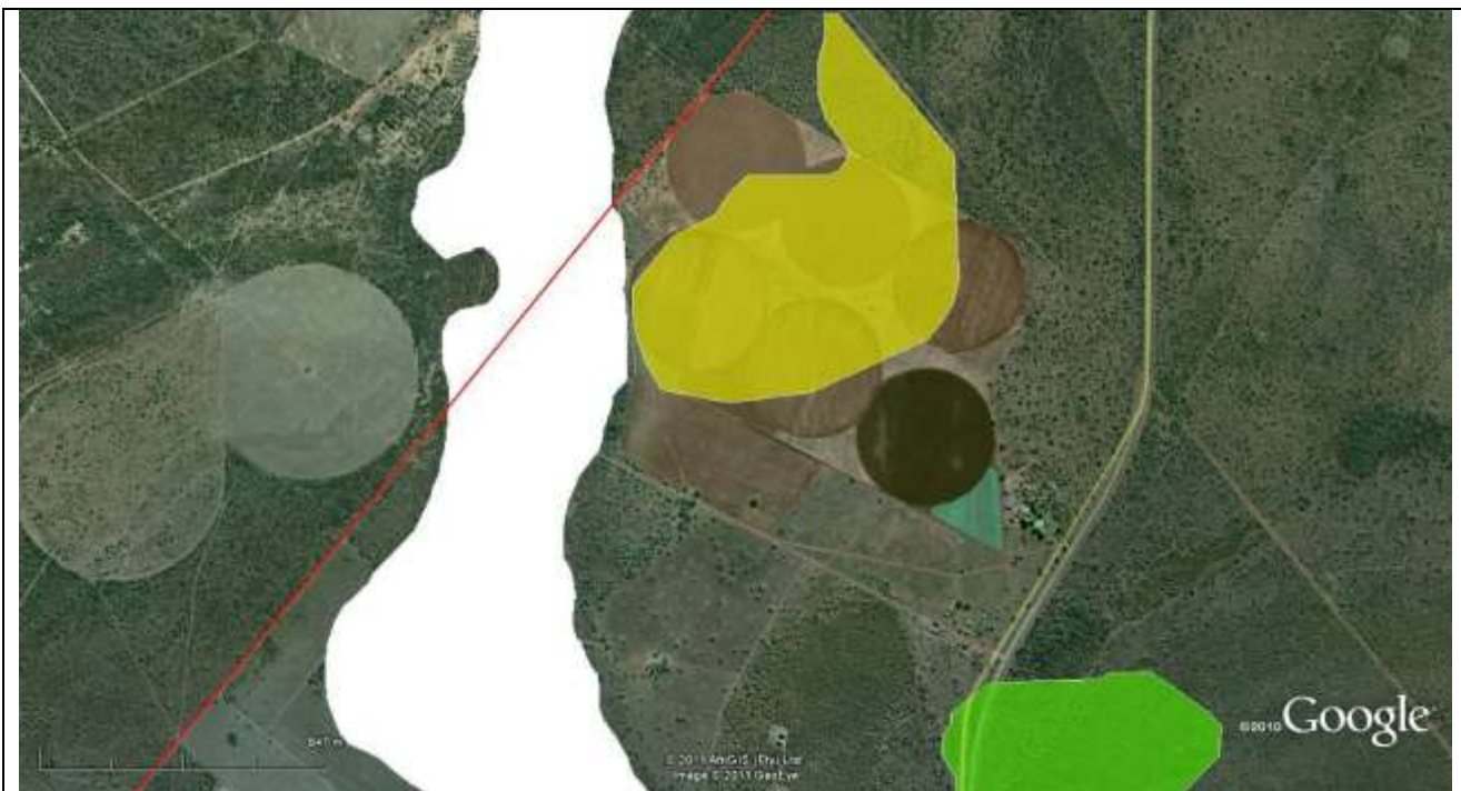
Figure 7-14: Position of North (yellow) and South (green) open cast pits in relation to the delineated wetland areas onsite. (WCS wetland delineation, 2011)
