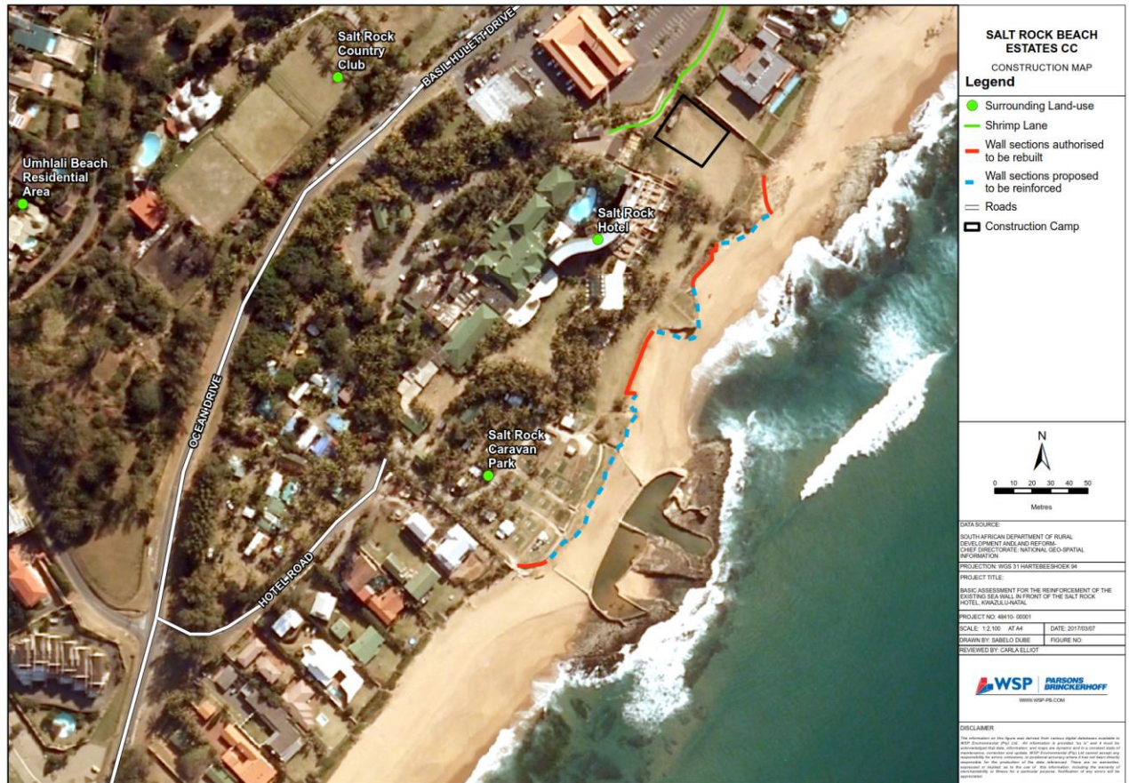
Figure 2 Preliminary proposed location of construction activities (WSP, 2018)
