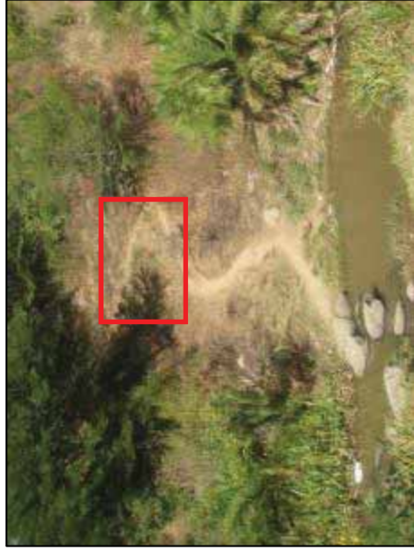
Figure 4: A view of the approximate point at which the bridge will begin on the southern banks (Red Square). Erosion could potentially result in this vicinity and the appropriate controls should be implemented to minimize erosion.
