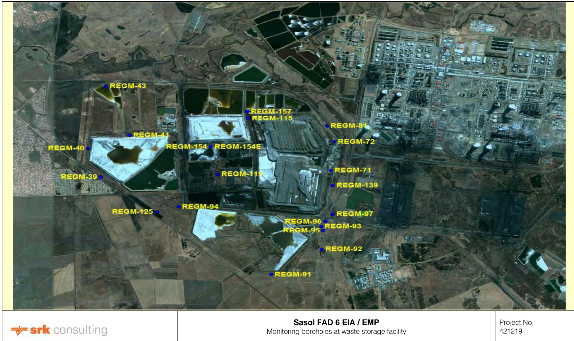
Figure 6-4: Monitoring boreholes at waste storage facilities
