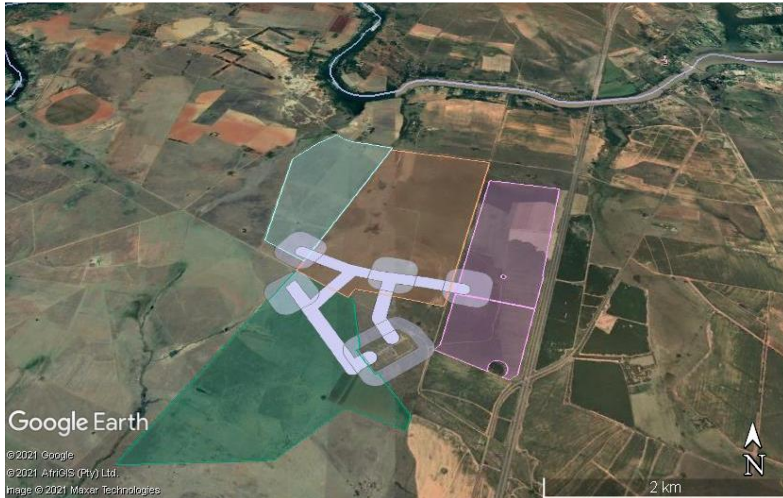
Figure 2: Google Earth map of the proposed Scaffell Cluster project for solar PV facilities and associated grid connection infrastructure. West (white area) is the Damlaagte Solar PV facility, the central (orange area) is the Scaffel Solar PV facility, the east (lilac area) is the Vlakfontein Solar PV Facility, and the southern section (green area) is the Ilikwa Solar PV Facility. Map supplied by HCAC/SLR.
