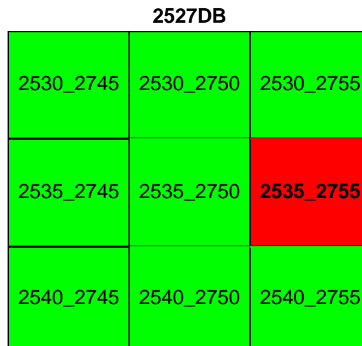
Figure 3: The 2527DB q.d.g.c. (15 minutes of latitude by 15 minutes of longitude, 15' x 15') is divided in nine smaller grids (5 minutes of latitude by 5 minutes of longitude, 5' x 5') of which each represent a pentad. The pentad in red represents the pentad in which the study site is situated.
