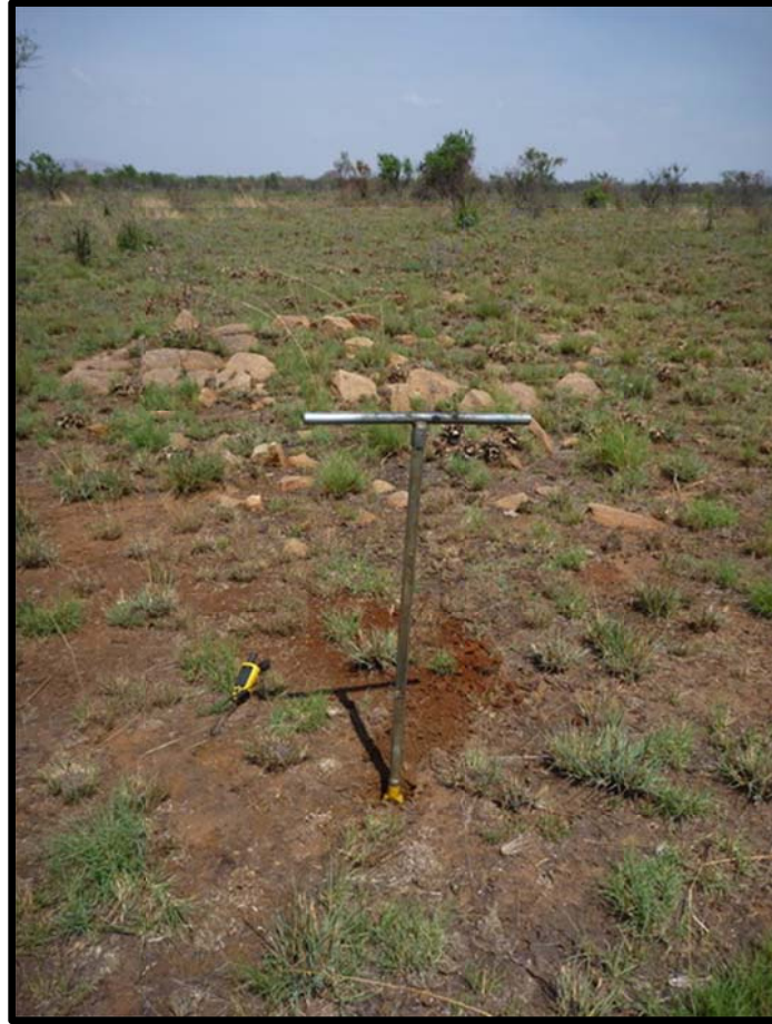
Figure 12 Abrupt changes in soil depth are noted in the area: The auger indicates a point where the soil is 90 cm deep while rock outcrops can be seen less than two meters away.
