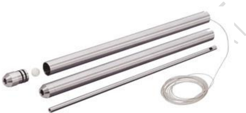
Figure 35: Stainless steel bailer, picture extracted from (Solist, n.d.). A bailer uses a simple ball check valve to seal a sample of the groundwater table at the bottom to raise it up.
