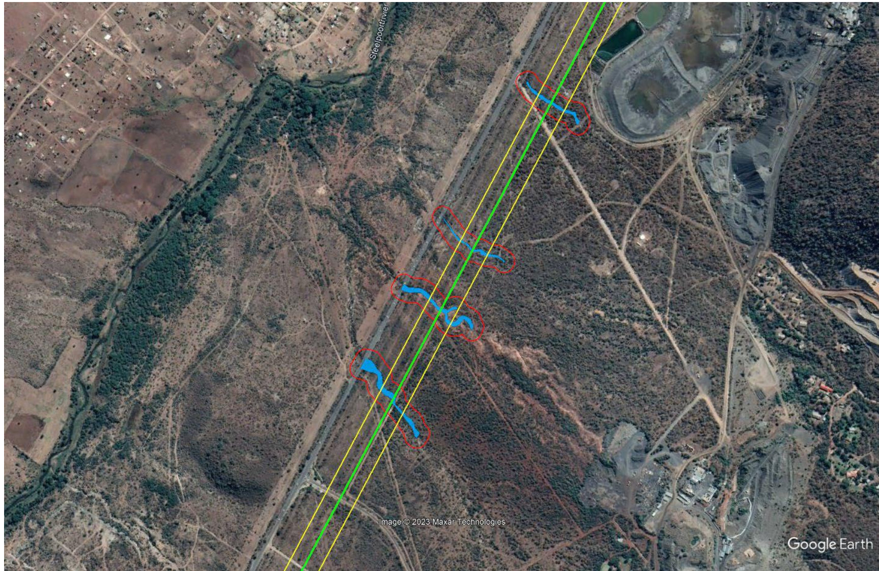
Watercourses and associated 32m buffer zones (Blue=Tributaries; Red=32m buffer zones; Yellow=100 m corridor; Green=Proposed Deviation)
