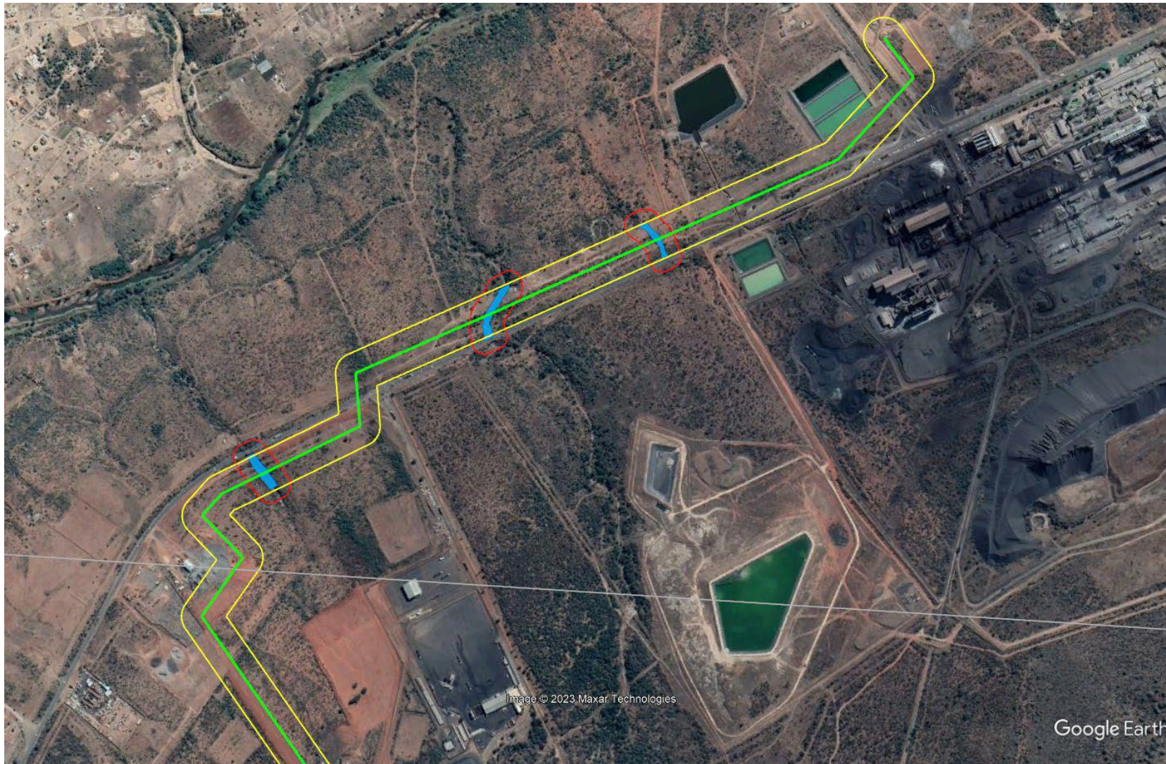
Watercourses and associated 32m buffer zones (Blue=Tributaries; Red=32m buffer zones; Yellow=100 m corridor; Green=Proposed Deviation)
