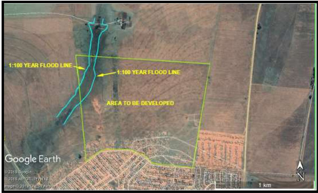
FIGURE 5: 1:100 Year Flood line of the Buisfontein Spruit
