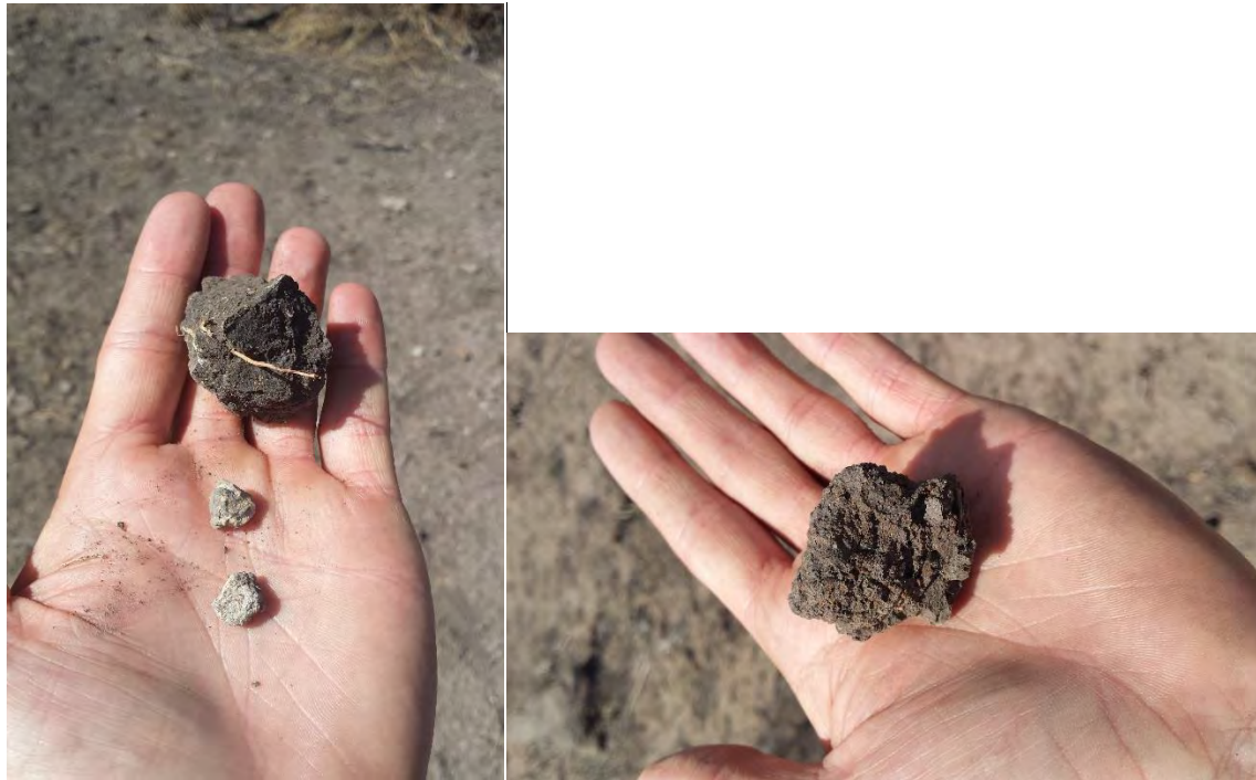
Figure 10. Dark Clay Soils with Calcretions (left) with Mottling at the Surface (right)
